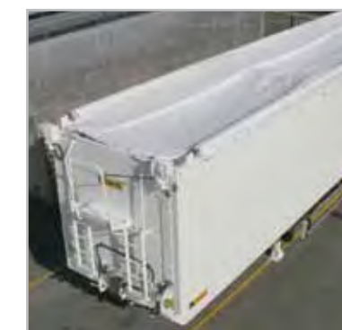
05 - Secured sheeting Electro-hydraulic control from the ground on front bulkhead.
