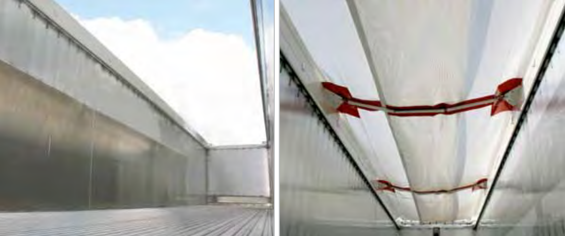
Inside aluminium plating 3 or 4 mm.
