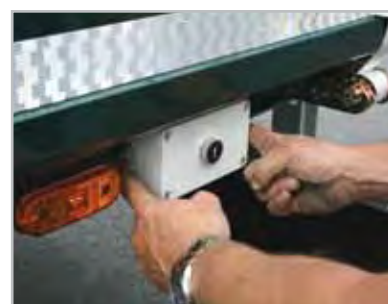
01 - Two-hand control Rear door secured with two-hand control and Buzzer alarm.
