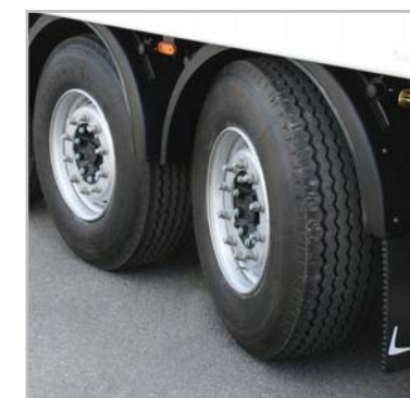
Rear self steering axle, Turn easier, greatly reducing tire wear, improving fuel economy.
