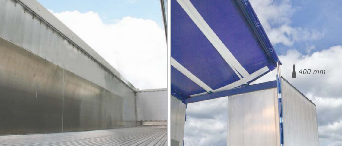
Inside aluminium plating 3 or 4 mm.
