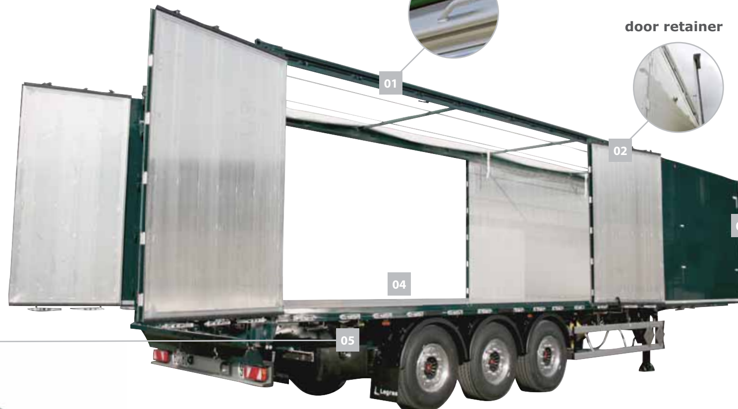
Roof sheet opens to preferred side With articulated sheet stops.
