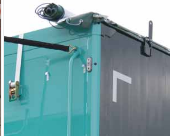
Roof sheet opens to preferred side With articulated sheet stops.
