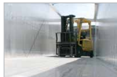
Robust floor, Will withstand use with 7 or 9 tonne forklift.
