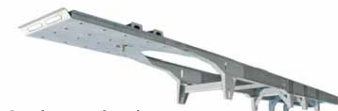
Continuous chassis Steel beams over the entire length of the trailer to avoid bending when the doors are open.
