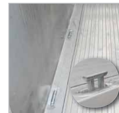
04 - Lashing rings, To secure the load (TUV certified).
