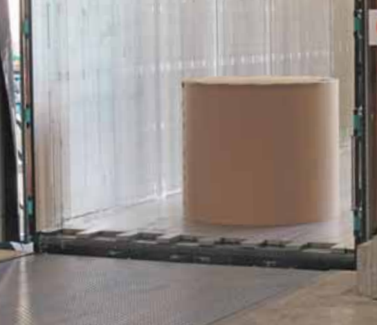
Smooth floor option for the transport of paper reels.
