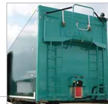
03 - Front bulkhead, With catwalk.
