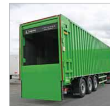
Guillotine door Aperture to receive the blade
