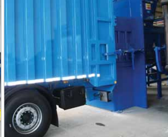
Coupling the trailer to the compactor
