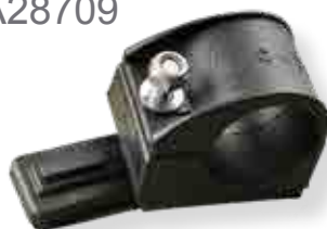
Kit support d'aile x 4 (pour 107A28692) Plastic mud wing stay (for 107A28692)
