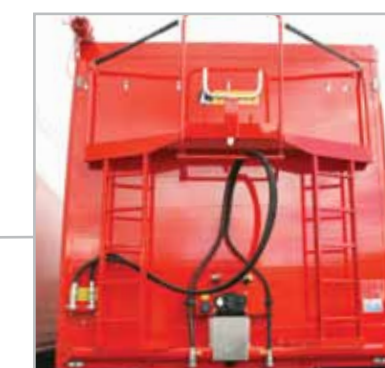
03 - Front bulkhead With catwalk and two ladders.
