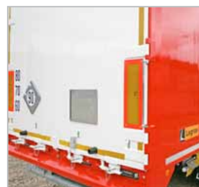
01 - Reinforced doors 4 integrated door through rod guide \varnothing 28.
